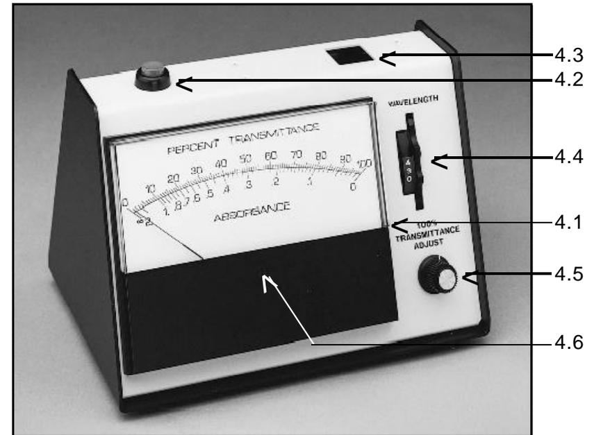
**4.1 Analog readout** - six inch meter face
